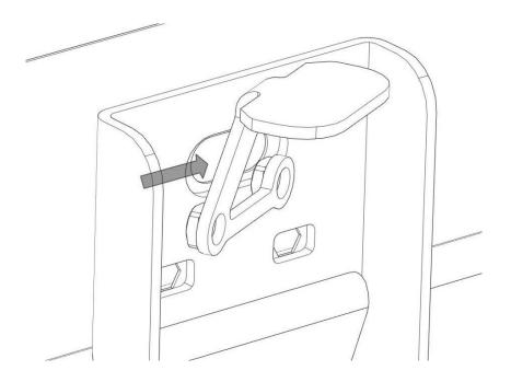
Figure 2 - INSTALLING THE FABFOURS Z-CLIP
