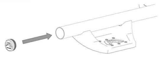
Figure 4 - INSTALLING THE FABFOURS SIDE STEP END CAPS
