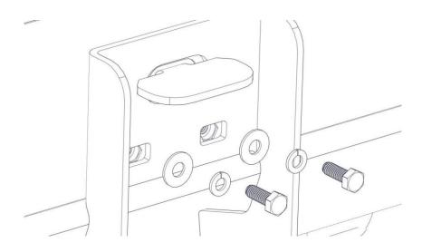
Figure 3 - ADDING THE HARDWARE TO THE FABFOURS Z-CLIP
