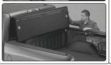
Slide the two front mounting bolts into the track on the underside of the Flex tonneau cover, one on each side. Place the Flex tonneau onto the mounting rails with the smallest panel towards the cab of the truck and with the front flap covering the bulkhead (front rail of the
